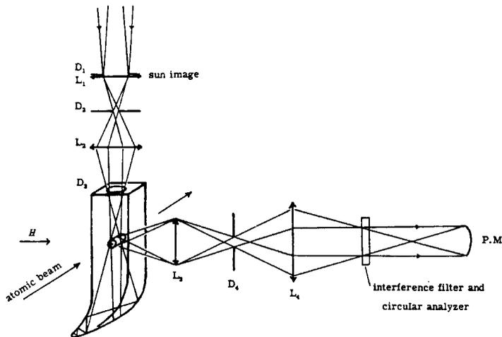
Figure 6. Set-up for the measurement of light resonance scattering with atomic beams.  $D_1$  is a blend for selecting a suitable part of the solar disc,  $D_2$  to  $D_4$  are blends against stray light and  $L_1$  and  $L_4$  are convex lenses; the magnetic field  $H$  is applied orthogonally to the axis of the atomic beam. *Source*: Blamont and Roddier (1964a), 438.
