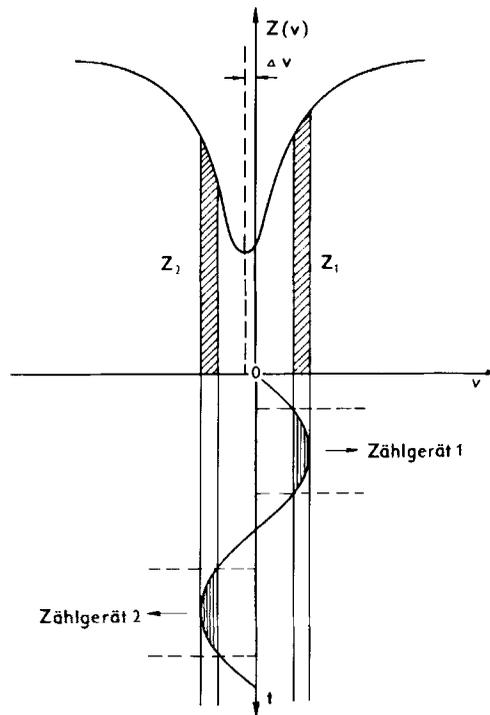
Figure 1. Asymmetry in the counting rates due to a shift  $\Delta\nu$  in the frequency of the absorption line. The source is moved sinusoidally with an amplitude correlating with the total line width. Source: Wegener (1966), 213.
