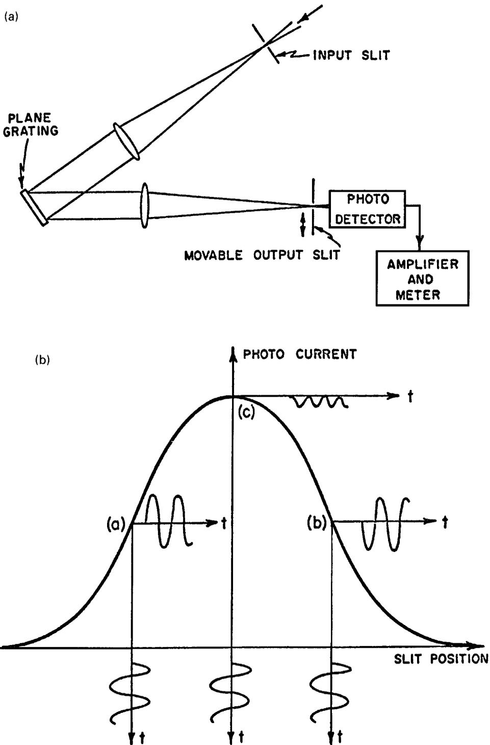
Figure 4. (a) Sketch of Brault's 1962 experimental set-up and (b) schematic illustration of the variation of the photoelectric signal with the slit's position relative to the maximum of an emission line. *Source*: Brault (1962), 27a.
