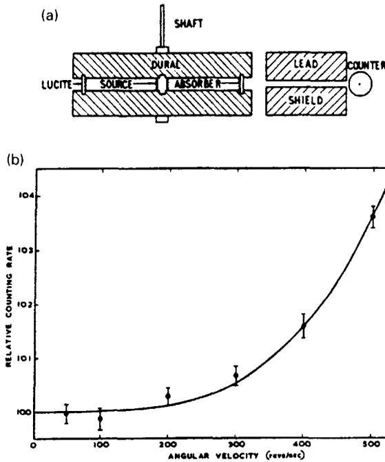
Figure 2. (a) Schematic diagram of the experiment by Hay *et al.* (1960) and (b) comparison of their data with the prediction from the principle of equivalency. *Source*: Hay *et al.* (1960).
